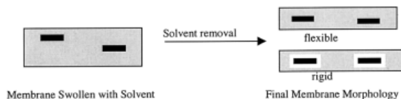
Figure 5 Hypothetical picture of mixed matrix material formation leading to formation of defects with rigid polymeric materials and defect-free materials with flexible polymers.
